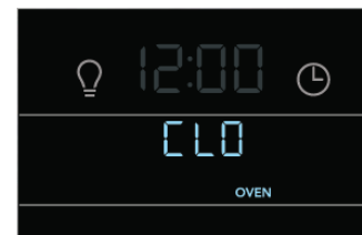
Figure 31: Message of open door that must be closed before oven can begin the clean cycle
