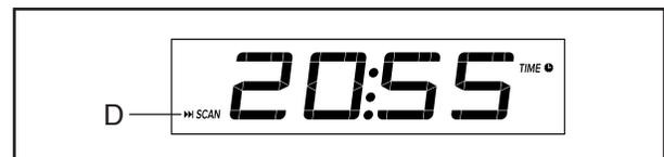
To manually advance the scan cycle, press the Scan button repeatedly.
