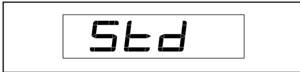
**Display Test**—This screen is intended to be used by service technicians to identify whether the display is working correctly.
