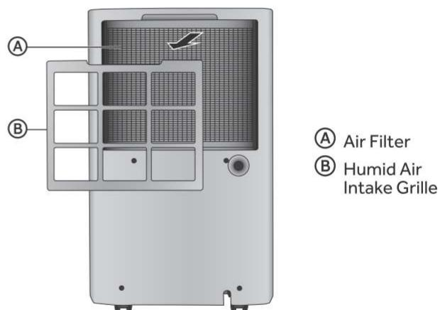
3. Wash or vacuum the dust from the air filters.
