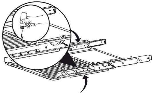
6. Extend and return the glide rack several times along the tracks to distribute the lubrication.
