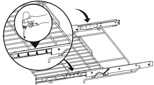
4. Extend and return the glide rack several times along the tracks to distribute the lubrication.
