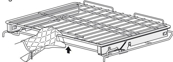
Figure 1 - Hold both upper and lower rack portions. Using both hands, lift up the front of the rack slightly and continue to pull the rack away from the oven (Figure 2). Be sure to grasp both upper and lower rack portions together when removing or handling the glide rack.
