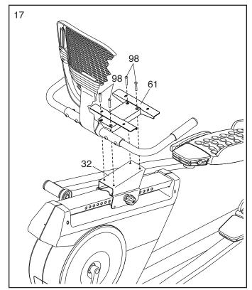
18. Attach the Seat (28) to the Seat Frame (61) with four M6 x 18mm Screws (97) (only two are shown); start all the Screws, and then tighten them.
