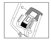
To insert a tablet or smart phone into the tablet holder (C), set the bottom edge of the tablet or smart phone in the tray. **Make sure that the tablet or smart phone** is firmly secured in the tablet holder. Reverse these actions to remove the tablet or smart phone from the tablet holder.
