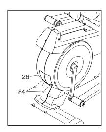
Next, locate the Reed Switch (60). Slightly loosen the two M4 x 16mm Screws (84).
