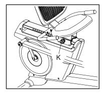
riage knob into an adjustment hole on the frame. Make sure that the carriage knob is securely inserted into an adjustment hole. Then, tighten the carriage knob.
