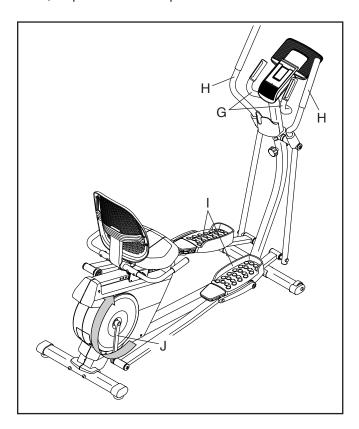
Push the pedals (I) until they begin to move with a continuous motion. Note: The crank arms (J) can turn in either direction. It is recommended that you move the crank arms in the direction shown by the arrow; however, for variety, you can turn the crank arms in the opposite direction.
