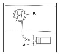
emergency, the key can be pulled from the console, causing the walking belt to slow to a stop. Test the clip by carefully taking a few steps backward; if the key is not pulled from the console, adjust the position of the clip.
