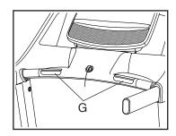
To measure your heart rate, stand on the foot rails and place your hands on the metal contacts—avoid moving your hands. When your pulse is detected, your heart rate will be shown. For the most accurate heart rate reading, continue to hold the contacts for about 15 seconds.
