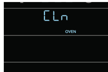
Figure 35: Clean lock icon blinks as door unlocks
