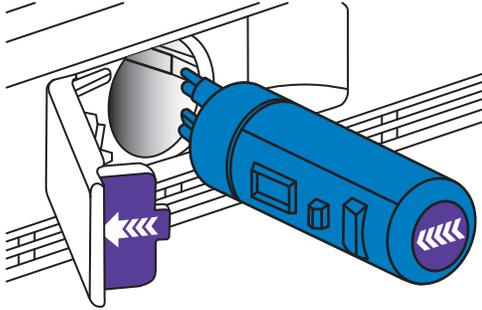
3. Take the new filter out of its packaging and remove the covers from the O-rings. Be sure the O-rings are still in place after the covers are removed.
