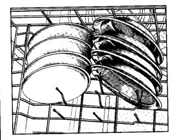
When loading glassware, leave a small space between each piece so they do not touch each other during the wash cycle. **Do not place** glasses over the tines. The hinged shelf can be used to stack two levels of cups, juice glasses, and other short items. Load small diameter items under shelf so water will reach upper tier. When the shelf is folded up, this area can be used for taller glasses, stemware, etc.
