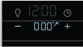
**Figure 25: Probe inserted and ready to set temperature**
