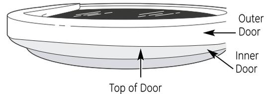
19. After reversing door, there will be a mismatch between the outer door and the inner door.
