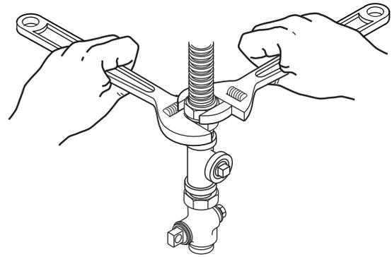
Tighten all connections using two adjustable wrenches. **Do not overtorque gas connections!**
