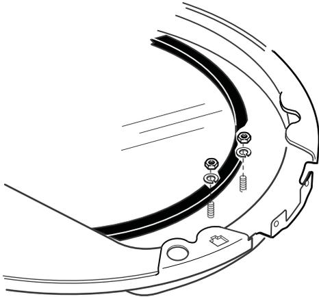
10. Remove the hinge assembly by removing the 2 machine screws (#8) that fasten it to the frame. Pull the hinge assembly out and set it aside.
