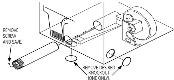
Detach and remove the bottom or left side knockout as desired. Remove the screw inside the dryer exhaust duct and save. Pull the duct out of the dryer. Protect sharp edges around the knockout and exhaust opening with the tape.
