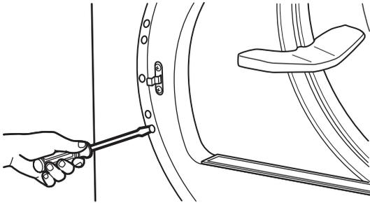
22. Switch the strike bracket and its cover to the opposite side by removing the screws; then reinstall both on the opposite side.
