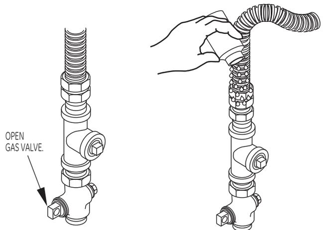
Check all connections for leaks with soapy solution or equivalent. Apply soap solution. **Leak test solution must not contain ammonia which could cause damage to the brass fittings.** If leaks are found, close valve, retighten the joint, and repeat the soap test.
