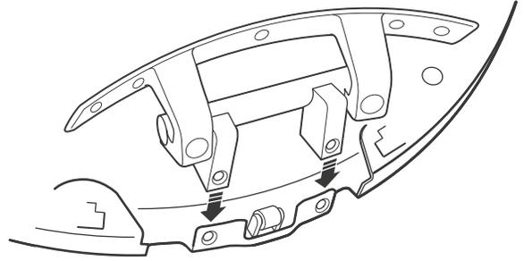
12. Loosely fasten the hinge assembly to the edge using 2 machine screws (#8).
