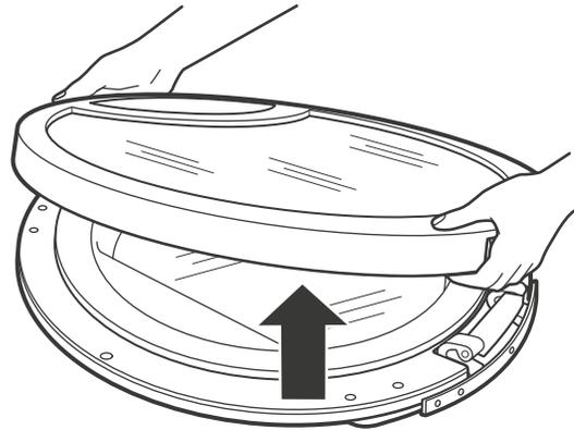
7. Unlock the 4 tabs on the plastic cover and separate the plastic cover from the frame.
