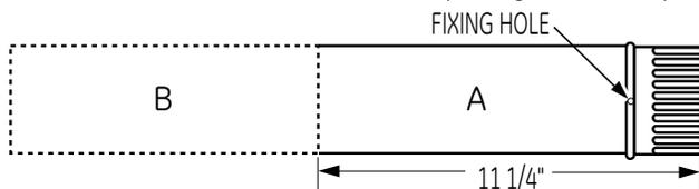
Cut the duct as shown and keep portion A.
