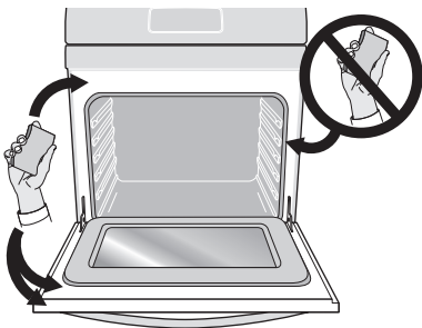
Figure 19: Clean around the oven door gasket
