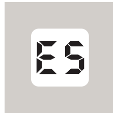
Evaporator coil sensor
