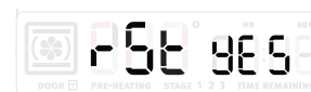
Figure 29: Display showing the options to reset to default (rSt yes) or to reject resetting to default (rSt no)
