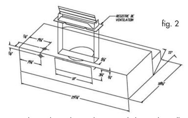
2. Once you have planned your ducting and electrical installation, remove the appropriate electrical knockouts on the back or top of the range hood, attach the damper frame and install a standard electrical cable clamp.
