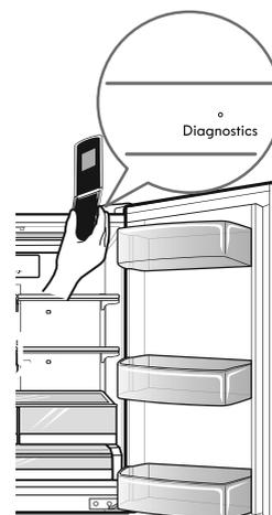
4. Press and hold the Freezer Temp button for three seconds while continuing to hold your phone to the speaker.
