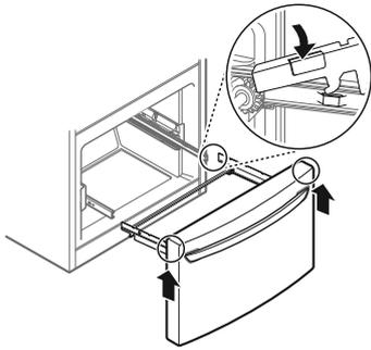
Lower the door into its final position and tighten the screws located on both sides.
