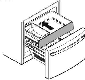
Replace the ice bin in the drawer. Insert the Durabase basket in the rail assembly.
