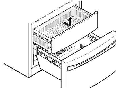
2. To install, slightly tilt up the front and insert the drawer into the frame and push it back into place.
