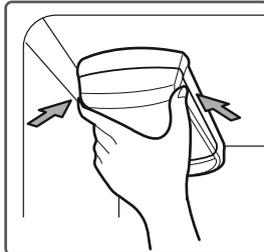
**NOTE:** Replacing the water filter causes a small amount of water (around 1 oz. or 25 cc) to drain. Place a cloth around the front end of the water filter cover to collect any leaking water. Hold the water filter upright, once it is removed, to prevent any remaining water from spilling out of the water filter.
