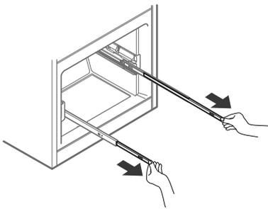
Grasp the drawer on each side and hook the drawer supports into the rail tabs located on both sides.
