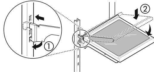
**CAUTION:** Make sure that shelves are level from one side to the other. Failure to do so may result in the shelf falling or food spilling.
