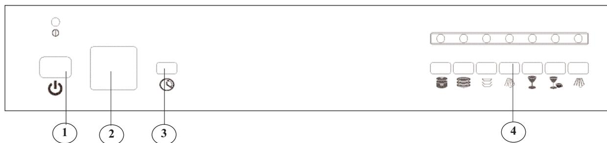
**1) ON/OFF Button:** Turns on/off the power supply.
