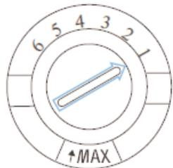
A measured amount of rinse aid is released during the final rinse. As with detergent, the amount of rinse aid needed for your dishes depends on the hardness of the water in your area. Too much rinse aid can result in lather or foaming and can cause cloudiness or streaks on your dishes. If the water in your area is very soft, you may not need rinse aid. If you do, you can dilute the rinse aid with an equal amount of water.
