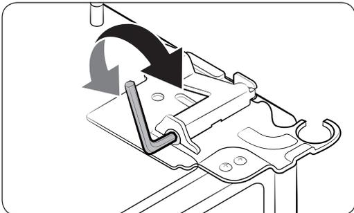
2. Use a 4 mm **Allen wrench** (not provided) to correct the door gap between two doors.
