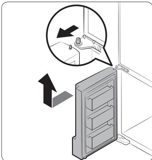
4. To prevent contact with the middle hinge, slightly tilt the door to the front, and then lift it up to remove.
