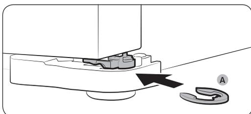
1. Check the height difference between the doors, and then raise and hold the lower door.
