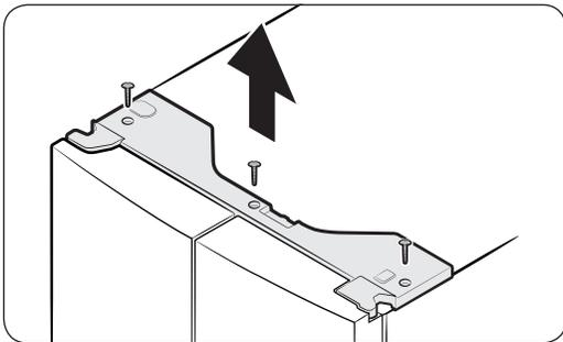
1. With the door closed, use a Phillips head screwdriver to remove the screws (x3) from the top cover. Pull up and remove the top cover with the connectors.
