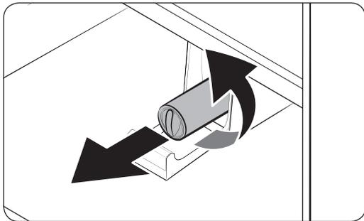
2. Turn the knob of the filter cartridge counter clockwise 90 degrees (1/4 turn). The filter cartridge unlocks.
