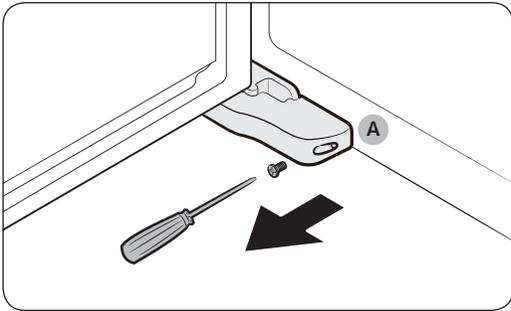
1. With the freezer door open, use a Phillips head screwdriver to remove the screw holding the **cover (A)** of the adjustable leg.
