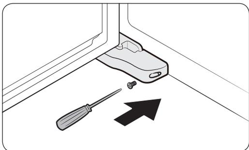
4. Attach the levelling foot cover using a Phillips head screwdriver. Be careful not to damage or step on the connectors.
