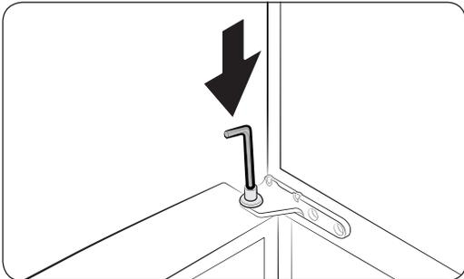
3. Locate the hinge shaft. While holding the door with one hand, use a flat-head screwdriver or wrench to press the shaft down. Make sure to hold the door to prevent the door from falling.
