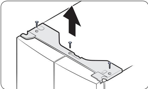
1. With the door closed, use a Phillips head screwdriver to remove the screws (x3) in the **top cover**. Then, carefully remove the **top cover** along with the wire connectors.
