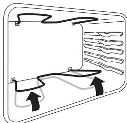
Figure 10: Lift bake element
