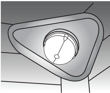
Figure 13: Wall oven Halogen light
