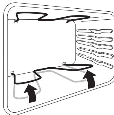
Figure 8: Lift bake element
