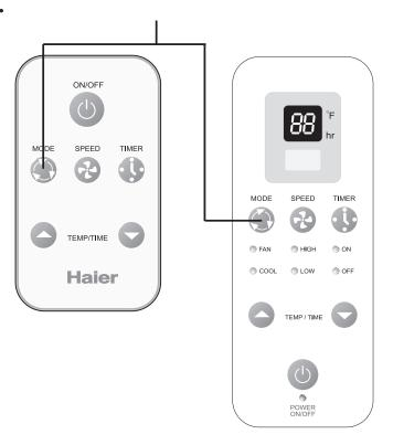
Once the function mode is decided you will have to set the fan speed. (See fig. #4) Every time you press the SPEED button, fan speed will change between LOW, HIGH
