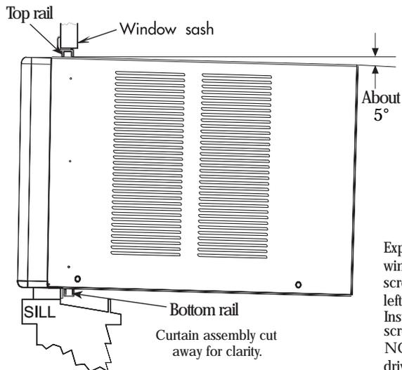
Expand both curtains to contact the window frame. Install four wood screws 31/32". Two in each upper right and left of the curtains. Install three wood screws 31/32" top mounting rail screws.
