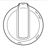
Electric igniters automatically light the surface burners when control knobs are turned to LITE. Before setting a control knob, place filled cookware on the grate. Do not operate a burner using empty cookware or without cookware on the grate.
