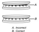
5. Turn on the burner. If the burner does not light, check cap alignment. If the burner still does not light, do not service the sealed burner yourself. Contact a trained repair specialist.
