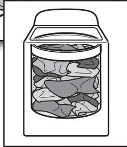
Load garments in loose heaps evenly around basket wall. For best results, do not pack the load tightly. Do not wrap large items such as sheets around the agitator; load them in loose piles around the sides of the basket. Try mixing different-sized items to reduce tangling.
