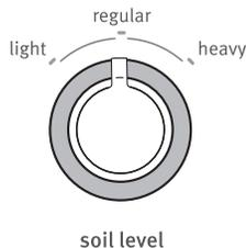
Once you select a cycle, select the soil level by turning the Soil Level knob to the desired setting.
