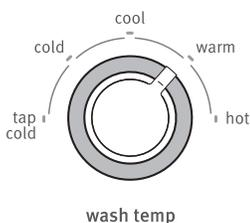
Once you select a cycle, select the wash temperature by turning the Wash Temp knob to the desired setting.
