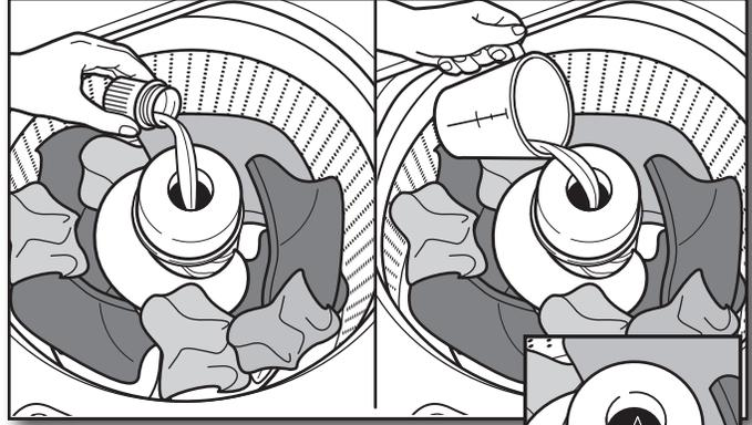
Pour a measured amount of liquid fabric softener into dispenser; always follow manufacturer's directions for correct amount of fabric softener based on your load size.
