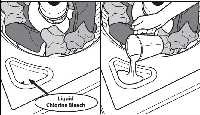
Do not overfill, dilute, or use more than 1 cup (236 mL). Do not use color-safe bleach or Oxi products in the same cycle with liquid chlorine bleach.
