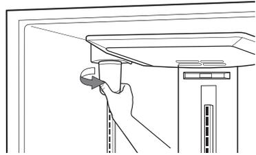
After replacing the filter, flush 2.5 gallons (9 liters) through filter before use (flush for approximately 5 minutes). Check the filter for leaks.
