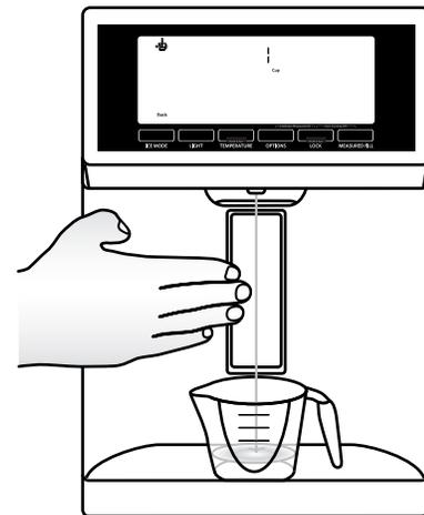
4. When 1 cup of water has been correctly dispensed into the measuring cup, press the MEASURED FILL button under the word “Confirm” to confirm the calibration.
