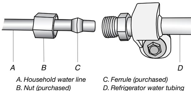
4. Install the water supply tube clamp around the water supply line to reduce strain on the coupling.
