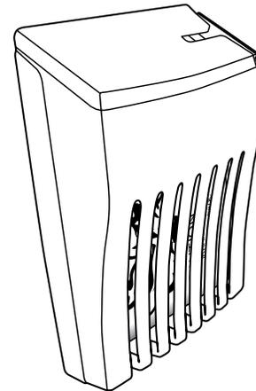
2. Open the housing by pulling up and out on the back.
