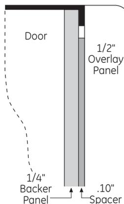
$$.250" + .10" + .50" = .850" \text{ Total Panel Thickness} \\ (0.635 \text{ cm} + 0.254 \text{ cm} + 1.27 \text{ cm} = 2.159)$$
