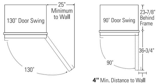
Allow 25" (63.5 cm) minimum clearance for a full 130° door swing. Allow 15" (38.1 cm) for pan removal.
