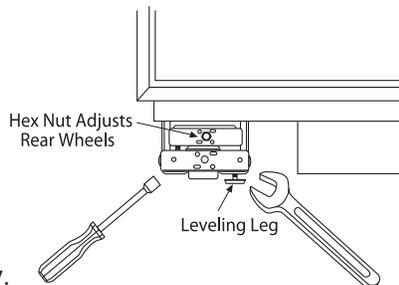
The rear leveling wheels and front leveling legs are limited to a maximum height adjustment of 1". If the installation requires more than 84-1/2" (214.63 cm) height, the installer should elevate the refrigerator on a sheet of plywood or runners. Cabinetry trim could also be added across the top of the opening to shorten the opening. If you attempt to raise the refrigerator more than 1" (2.54 cm), you will damage the front leveling legs and the rear leveling wheels.
