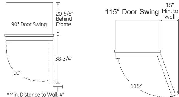
For a 90 degree door swing, allow 4" (10.16 cm) min. clearance to wall. If the 90 degree door stop position is used, pan access is maintained, but pan removal is restricted
