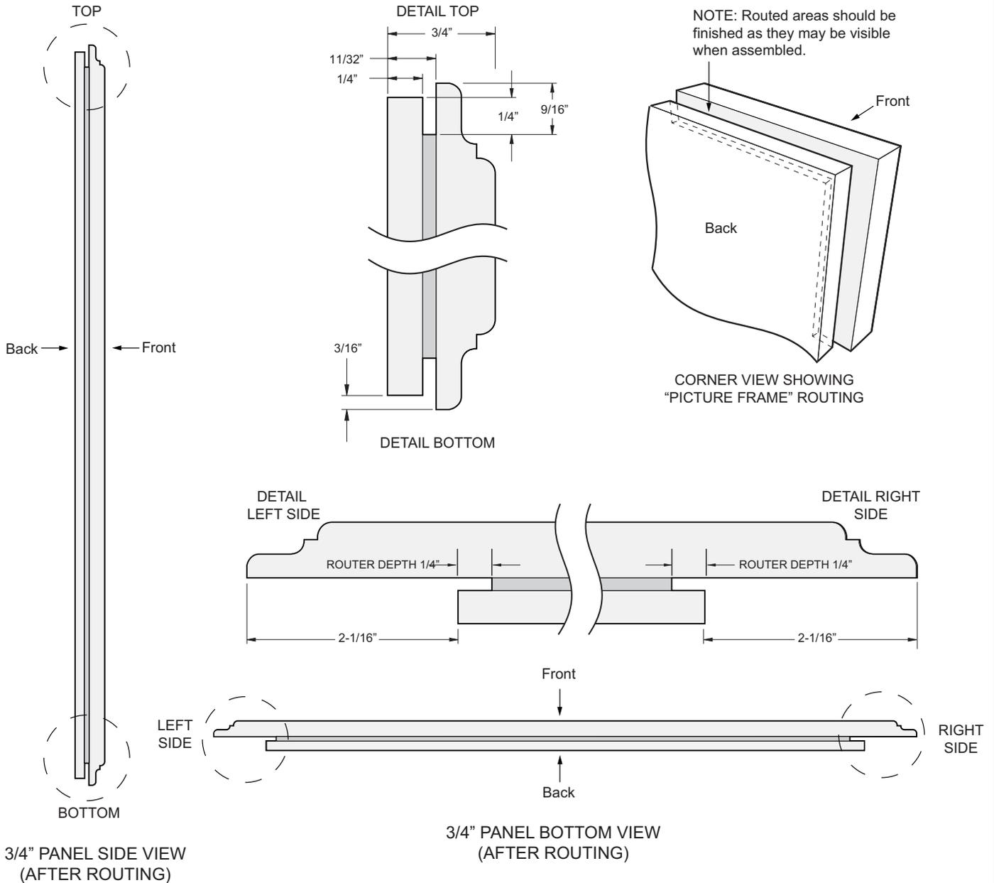
**NOTE:** For panels constructed with rails and stiles (5-panel), the minimum width is 3" (7.62 cm) for rails and 4" (10.16 cm) for stiles.
