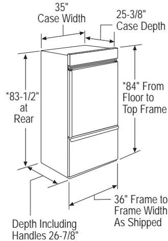
\* Shipping height. The refrigerator can be adjusted to fit into a cutout that is 84-1/2" (214.63 cm) max. height. Note that the top case trim at the front is 1/2" (1.27 cm) higher and will overlap upper cabinetry or soffit. Use leveling legs and wheels for a maximum 1" (2.54 cm) height adjustment.
