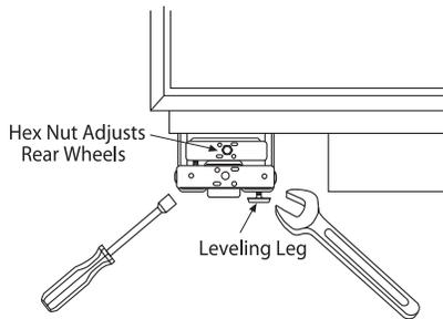
The rear leveling wheels and front leveling legs are limited to a maximum height adjustment of 1" (2.54 cm). If the installation requires more than 84-1/2" (214.63 cm) height, the installer should elevate the refrigerator on a sheet of plywood or runners. Cabinetry trim could also be added across the top of the opening to shorten the opening. If you attempt to raise the refrigerator more than 1" (2.54 cm), you will damage the front leveling legs and the rear leveling wheels.
