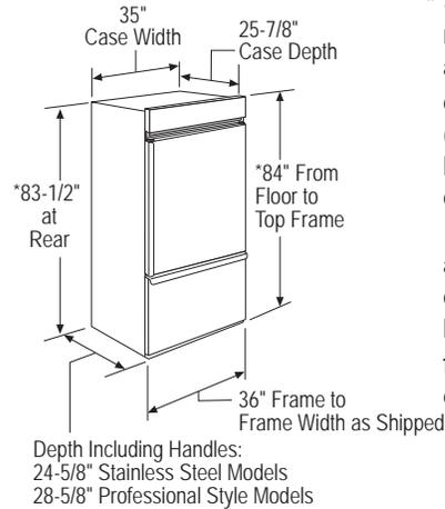
\* Shipping height. The refrigerator can be adjusted to fit into a cutout that is 84-1/2" (214.63 cm) max. height. Note that the top case trim at the front is 1/2" (1.27 cm) higher and will overlap upper cabinetry or soffit. Use leveling legs and wheels for a maximum 1" (2.54 cm) height adjustment.
