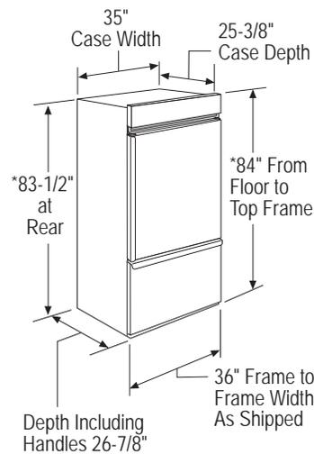
\* Shipping height. The refrigerator can be adjusted to fit into a cutout that is 85" (215.9 cm) max. height. Use leveling legs and wheels for a maximum 1" (2.54 cm) height adjustment.
