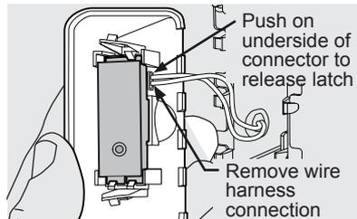
Push on underside of connector to release latch
