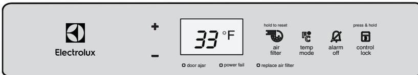
To adjust the temperature setting, press the UP (+) key for warmer temperature and DOWN (-) key for colder temperature on the control panel. Allow several hours for the temperature to stabilize between adjustments. The unit can be adjusted between 33°F (1°C) and 46°F (8°C). By pressing the TEMP MODE key, the temperature display will toggle between °F to °C.
