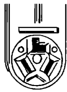
three-wire receptacle (10-30R) Figure 4
