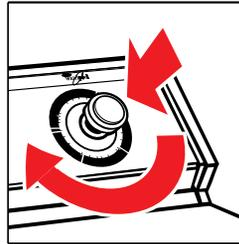
7. Pull out the Cycle Control Knob to start the washer.
