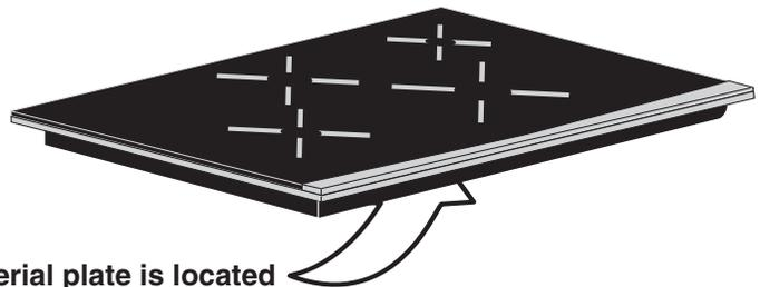
Serial plate is located under the burner box of cooktop.
