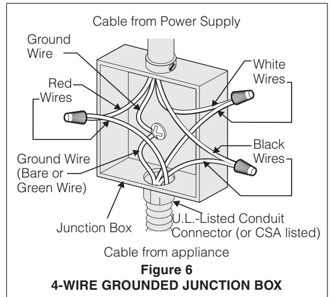
**⚠ WARNING** If connecting to a 4-wire power supply cable electrical system, the appliance frame connected ground wire **MUST NOT** be connected to the neutral wire of the 4-wire electrical system.
