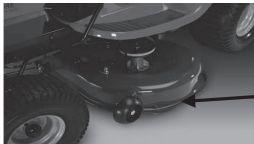
Stamped Deck Shell below, NOT reinforced
