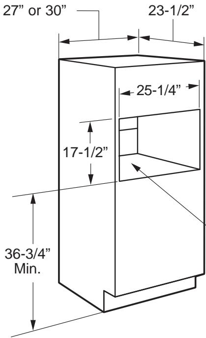
Construct solid bottom - Min. 3/8" plywood supported on all four sides. Must be able to support weight of oven and contents.
