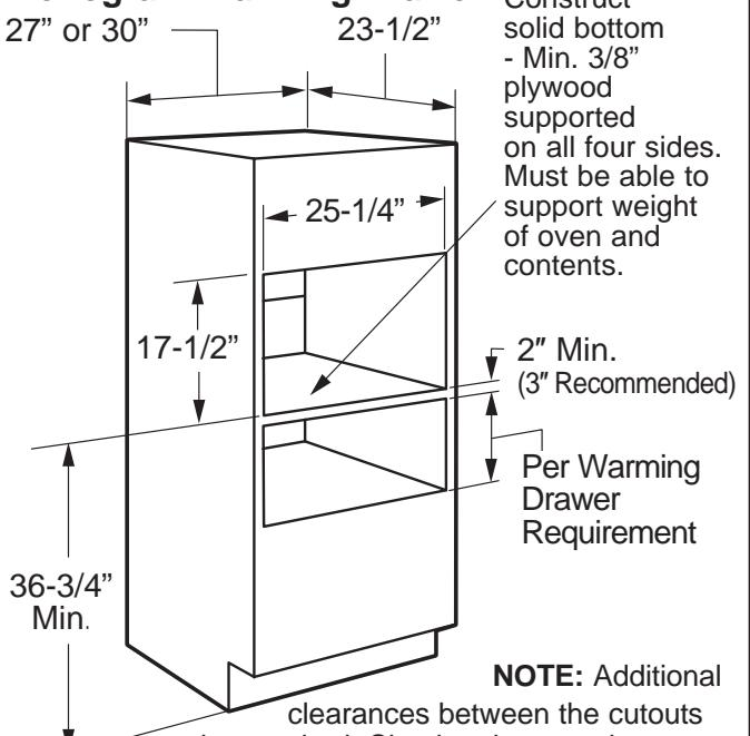
**NOTE:** Additional clearances between the cutouts may be required. Check to be sure the oven supports above the Warming Drawer location does not obstruct the required interior depth and height. See Warming Drawer installation instructions for details.
