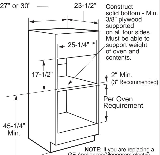
**NOTE:** If you are replacing a GE Appliances/Monogram electric double oven with the combined installation of an Advantium 120 and a single oven, use the dimensions shown. The middle rail separating the two openings may need to be larger than the 2" minimum shown.
