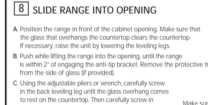
To reduce the risk of tipping the range, the range must be secured by a properly installed anti-tip bracket. See installation instructions shipped with the bracket for complete details before attempting to install.
