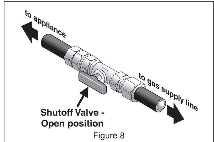
Once regulator is in place, open the shutoff valve in the gas supply line. Wait a few minutes for gas to move through the gas line.
