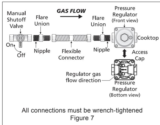
Assemble the flexible connector from the gas supply pipe to the pressure regulator in the following order:
