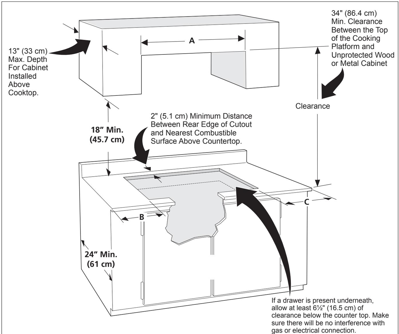
**⚠ CAUTION** To eliminate the risk of burns or fire from reaching over heated surfaces, cabinet storage space located above the cooktop should be avoided. If cabinet storage is provided, risk can be reduced by installing a range hood that projects horizontally a minimum of 5" (12.7 cm) beyond the bottom of the cabinets.
