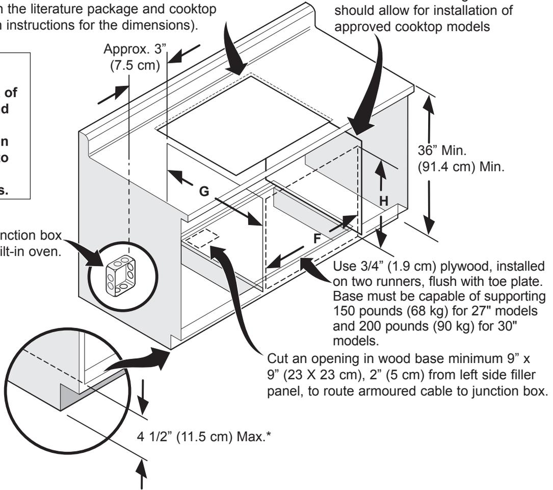
\* If no cooktop is installed directly over the oven unit, 5" (12.7 cm) maximum is allowed above the floor.
