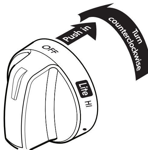
Figure 7: Correct way to set burners
