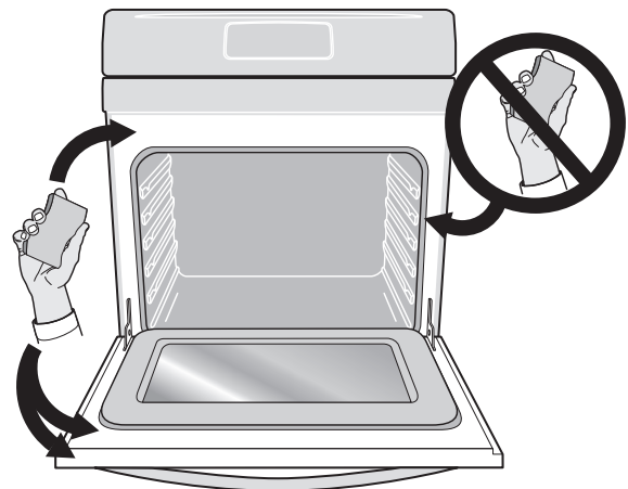
Figure 14: Clean around the oven door gasket
