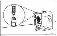
Align the pins on the stir tower shaft with the slots on the flip-and-stir wand. Press the wand up and rotate counterclockwise to lock into place.
