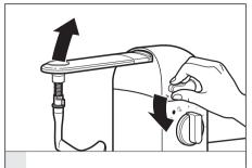
Raise the stir arm by pressing down on the release lever.
