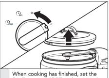
Stir Tower to 0 (OFF) and remove the 3 lid from the pot using a hot pad or oven mitt.
