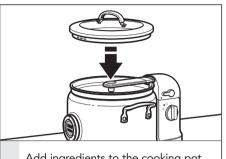
Add ingredients to the cooking pot, align the cutout in the multi-cooker 1 lid with the stir arm and cover the cooking pot.
