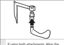
If using both attachments: Align the tab on the top of the flip-and-stir wand with the groove on the side scraper and slide into place.
