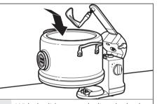
With the lid removed, align the back of the Multi-Cooker with the front of the Stir Tower. Make sure the Stir Speed selector is set to 0 (OFF) position before placing the Multi-Cooker onto the easy connect power port on the stir tower base.
