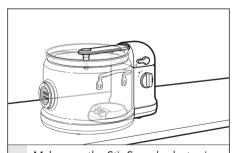
Make sure the Stir Speed selector is set to the 0 (OFF) position. Place the stir tower on a sturdy, level surface such as a countertop, with enough space for the Multi-Cooker.
