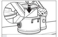
Place the cooking pot in the Multi-Cooker, aligning the notch in the cooking pot with the stir arm.
