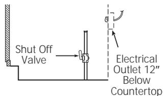
Install a manual shut-off valve in the gas line in an easily accessible location outside the cooktop. Be sure you know how and where to shut off the gas supply to the cooktop. Install the electrical outlet 12" below the countertop.
