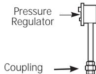
To reduce the likelihood of gas leaks, apply teflon tape or a thread compound approved for use with Propane (LP) or Natural gases to all threaded connections.
