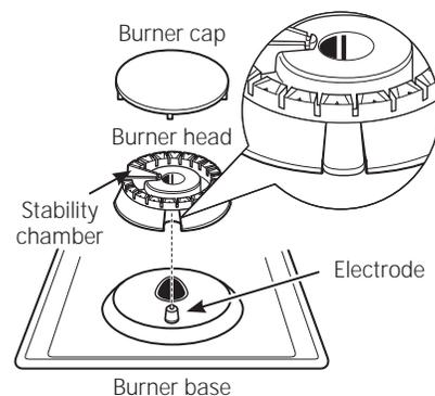
Make sure the hole in the burner head assembly is positioned over the electrode and that the burner head is fully inserted inside the burner base. A small gap between the base and head is normal.
