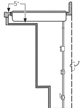
**NOTE:** The enclosure must be made of wood material. Also, an access panel is required for the electrical outlet, pressure regulator, shut-off valve, hold-down brackets, and service.
