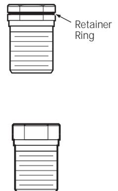
**NOTE:** For orifices that do not have a spring-loaded retaining ring, use pliers to hold the orifice in position during initial thread engagement or final removal to avoid dropping the orifice in the cooktop. Then use the nut driver to tighten or loosen.
