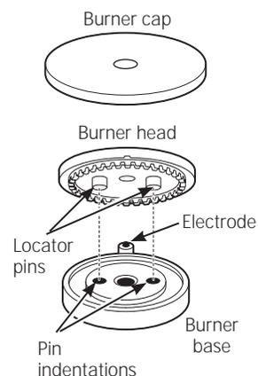
Make sure the slot in the burner head is positioned over the electrode.
