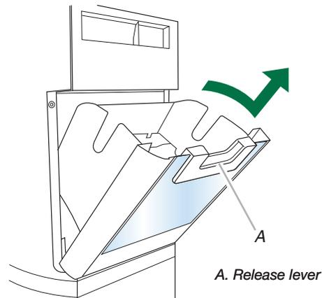
**NOTE:** It is not necessary to flip the ice maker On/Off switch to the OFF (down) position when removing the storage bin. The storage bin sensor, located on the right wall of the freezer door, stops the ice maker from producing ice if the door is open or the storage bin is removed.
