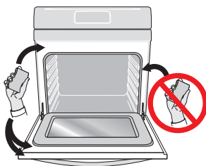
Figure 24: Clean around the oven door gasket
