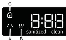
When delay is selected, the fully lit display will show the number of hours to delay and an "H" for hour.
