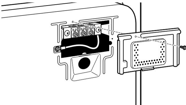
Remove hold-down screw and terminal block cover.
