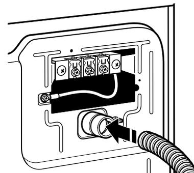
Put direct wire cable through the strain relief. The strain relief should have a tight fit with the dryer cabinet and be in a horizontal position. Tighten strain relief screw against the direct wire cable.
