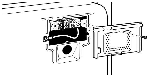
Remove hold-down screw and terminal block cover.
