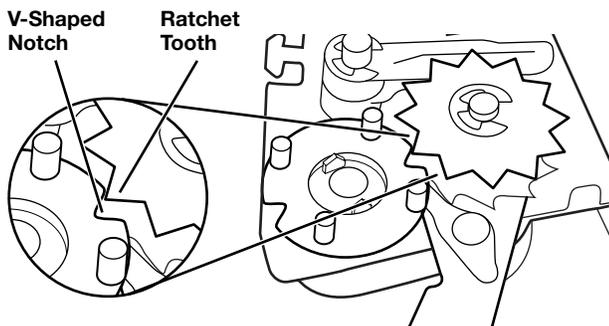
4. Insert a narrow, flat-blade screwdriver under the timing cam near the clock shaft. Gently lift cam straight up and off shaft, making sure that the V-shaped notch clears the ratchet tooth.
