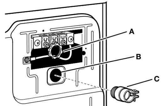
Unscrew the removable conduit connector (A) and any screws from a  $\frac{3}{4}$ " (19 mm) UL listed strain relief (UL marking on strain relief). Put the threaded section of the strain relief (C) through the hole below the terminal block opening (B). Reaching inside the terminal block opening, screw the removable conduit connector (A) onto the strain relief threads.
