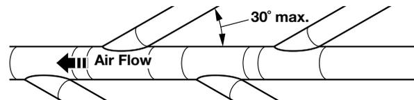
The maximum angle of each vent entering the main vent should be no more than 30°.
