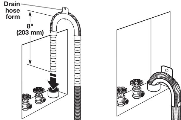
6. For floor drain installations, you will need to remove the drain hose form from the end of the drain hose. You may need additional parts with separate directions. See "Tools and Parts."
