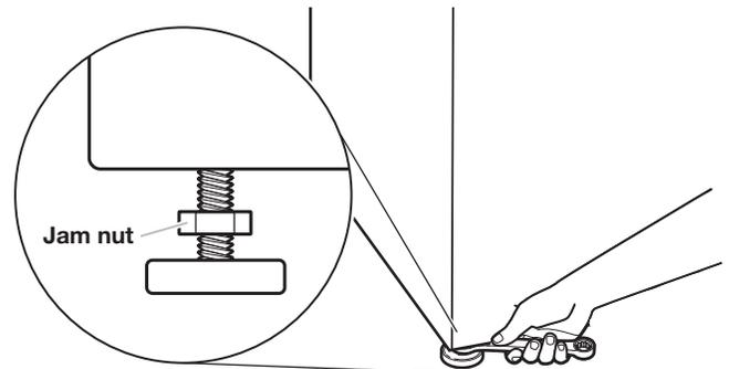
3. When washer is level, use a 9/16" or 14 mm open-end or adjustable wrench to turn jam nuts counterclockwise on leveling feet tightly against washer cabinet.
