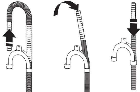
7. The floor drain system requires a siphon break that may be purchased separately. The siphon break (Part Number 285320) must be a minimum of 28" (710 mm) from the bottom of the washer. Additional hoses might be needed.
