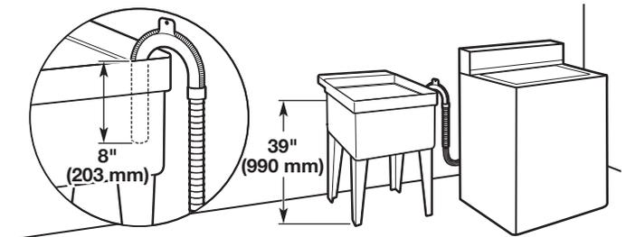
Minimum capacity: 20 gal. (76 L). The top of the laundry tub must be at least 39" (990 mm) above floor.
