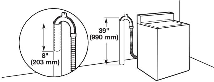
Minimum diameter for a standpipe drain: 2" (51 mm). Minimum carry-away capacity: 10 gal. (38 L) per minute. Top of standpipe must be at least 39" (990 mm) high; install no higher than 96" (2.44 m) from bottom of washer.
