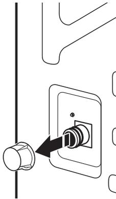
2. If clamp is not already in place on elbow end of drain hose, slide it over end as shown.
