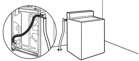
Floor drain system requires a Siphon Break Kit (Part Number 285320). Minimum siphon break: 28" (710 mm) from bottom of washer. Additional hoses may be needed.
