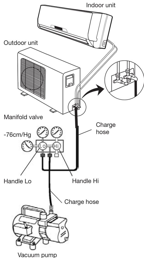
display in the pressure indicator is a little higher than the atmosphere pressure. This procedure verifies if the refrigerant goes through the tubes correctly.
