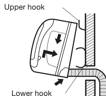
3. Piping can easily be made by lifting the indoor unit with a cushioning material between the indoor unit and the wall. Get it out after finish piping.
