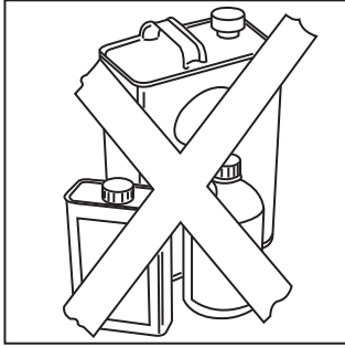
Fig. 4 – NO combustible materials near furnace
