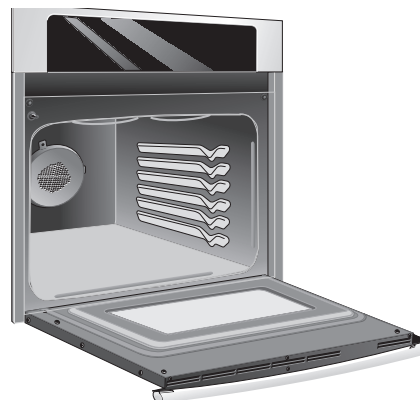
Figure 36: Door at horizontal position
