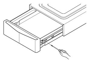
4 Remove three (3) screws on the drawer.
