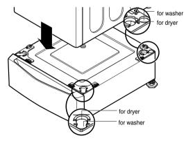
**NOTE:** The legs on the washer and dryer are not the same, so the recesses in the brackets on top of the pedestal are elongated. See the drawing above to identify the different locations for the washer and dryer legs. If the legs are not in the proper locations, the machine will not align properly and cannot be anchored to the pedestal.
