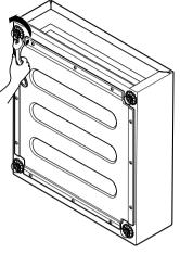
**9** Remove four (4) screws (two on each side) on both side of slide.
