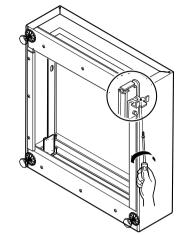
8 Remove twelve (12) screws on the bottom of the pedestal.
