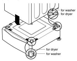
A Make sure the holes on the pedestal align with the holes in the appliance, then install 4 screws at each corner to securely attach the appliance to the pedestal.
