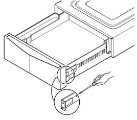
3 Pull up the drawer to disassemble.
