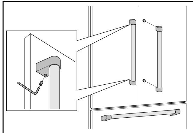
2. Loosen the setscrew counter-clockwise a quarter-turn at a time. Repeat for each of the setscrews.
