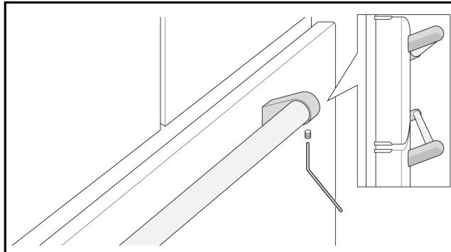
9. Once both setscrews have been partially tightened as instructed in the previous steps, fully tighten both setscrews.
