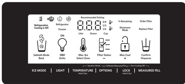
**IMPORTANT:** The display screen on the dispenser control panel will turn off automatically and enter Sleep mode when the control buttons and dispenser paddles have not been used for 2 minutes or more. Press any control button to reactivate the display screen. The home screen will appear as shown.
