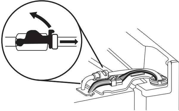
3. Disconnect the wiring plug located on top of the door hinge.
