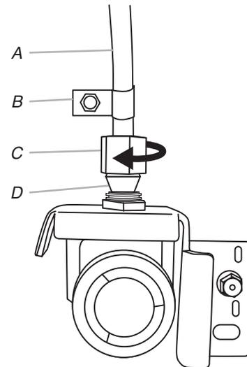
3. Turn on water supply to refrigerator and check for leaks. Correct any leaks.
