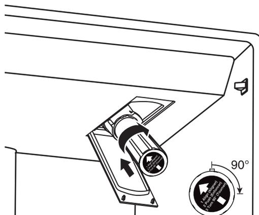
6. While the compartment door is still open, lift the filter up into the compartment. Then, close the filter compartment door completely.
