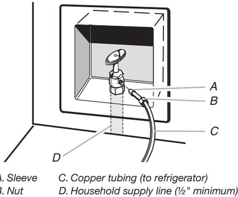
4. Now you are ready to connect the copper tubing to the shutoff valve. Use ¼" (6.35 mm) OD soft copper tubing to connect the shutoff valve and the refrigerator.
